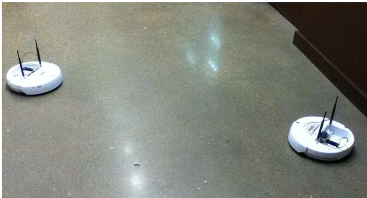
Figure 8: One configuration of iRobot Creates used to collect real-world RSSI data. Many configurations of walls and obstacles between the robots were used in the data collection.
